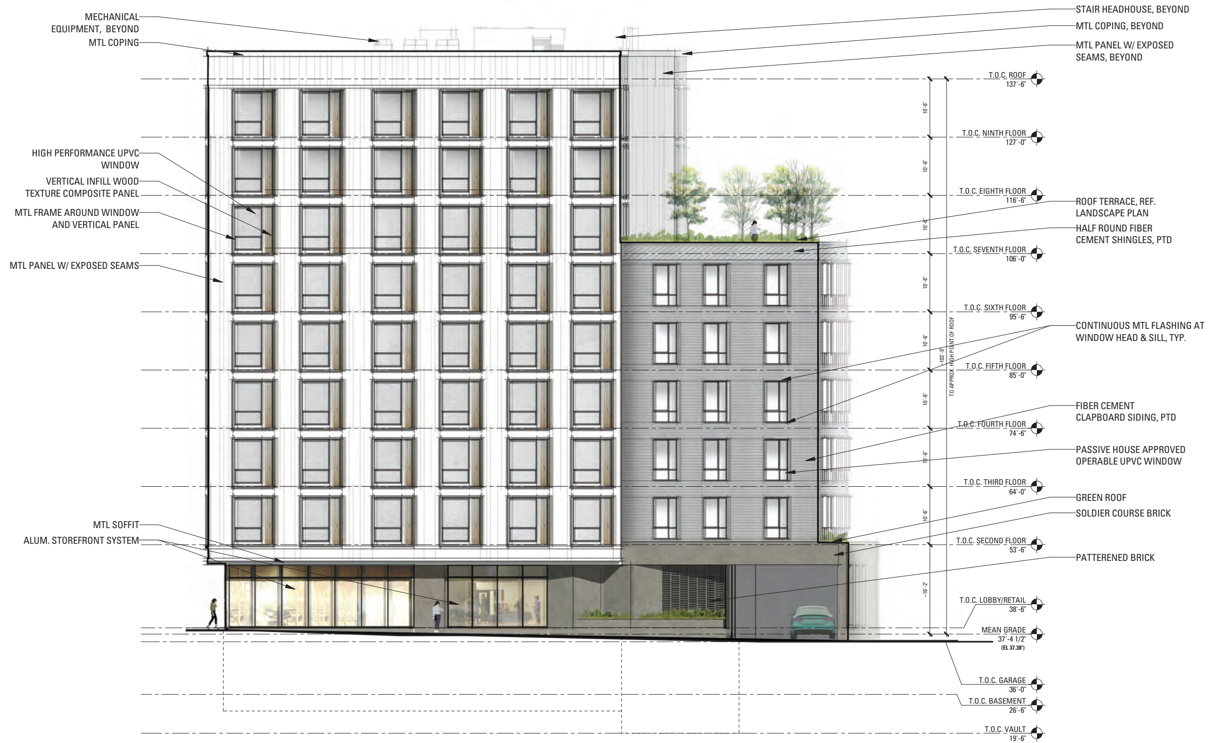
1 BUILDING ELEVATION - WEST SCALE: 1/8" = 1'-0"
